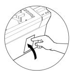
3. Swing the Rejected Card Box Door and press the top. An audible "click" signals the locked position.
